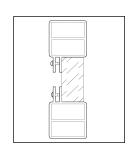
Attachment for insulated core panel up to 1.375" thick.
