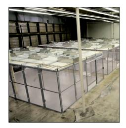
AirLock is designed to keep assembly areas free of contaminants and dust. Walls and anodized aluminum frames wash down quickly and easily.
