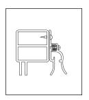
Typical softwall attachment with Simplex Hookbead mounting bar.
