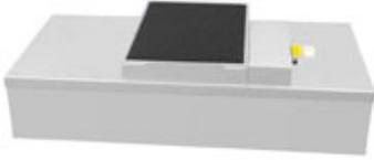
As one of the most innovative Fan Filter Units (FFU) available, the MAC 10 Original combines low watts, low sound and a low profile. The MAC 10 Original sound level is only 49 dBA, and by operating at 170 watts, the MAC 10 Original uses less energy, resulting in lower operating costs. Plus, the unit still measures less than 13 in. (330 mm).
